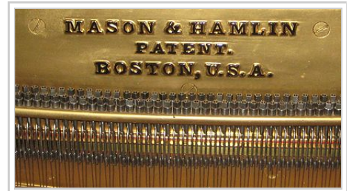
Detail of an 1894 Mason & Hamlin upright piano, showing the "screw stringer" apparatus.
